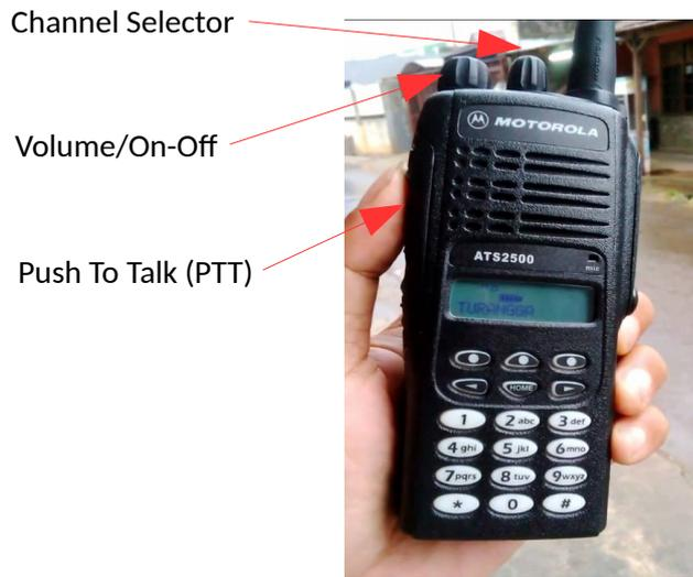
The radios in use at Blazing Swan in 2017 and 2018 were Motorola ATS2500's. We will likely be using the same radios this year but this is not guaranteed. These radios have been programmed to make them as simple as possible to use.
